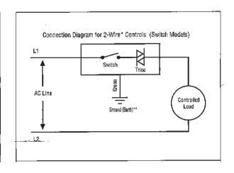
\*Ground wire is not counted when designating 2, 3 or 4 wire controls.
