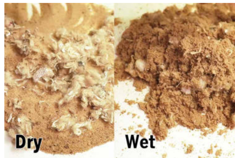
Left: The dry materials can't mix together. Footing products rise to the top of the surface. Right: Water binds the sand and textiles together and add a structure to the footing.
