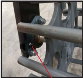
Fig 89. Location of Grease Fitting on Wheel Hub Assembly.
