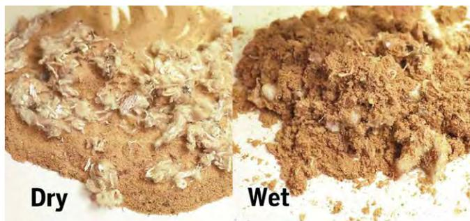
**Left:** The dry materials can't mix together. Footing products rise to the top of the surface. **Right:** Water binds the sand and textiles together and add a structure to the footing.
