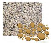
One of the first things we analyze in an equestrian arena is the gradation of the sand particles. This refers to the range of particle sizes. A well-graded sand will have a combination of different sized particles. The variation of small particles fills the voids between the larger particles, stabilizing the surface from shifting and rolling.
