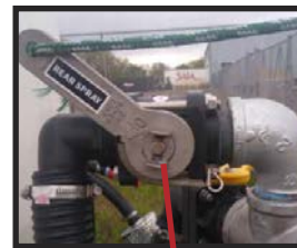
Silver tab on valve is perpendicular to plumbing when valve is closed.
