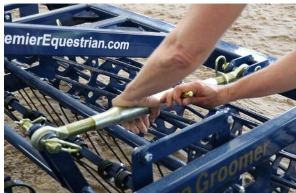
Rotate turnbuckles to raise and lower tine sets. Set the lock to hold the turnbuckles the position.
