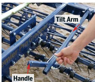
Remove the pin to adjust tilt arm
